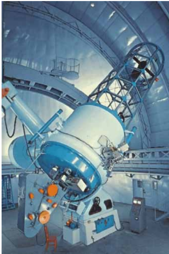
DAVID DUNLAP OBSERVATORY TELESCOPE. Seventy-four feet tall, weighing 23 tons and sporting a 2 ton mirror, the David Dunlap Observatory telescope is well worth the trip just to look at. Thanks to the Royal Astronomical Society of Canada volunteers you can also look through it if the night is clear.
